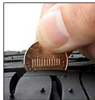
A covered Lincoln Memorial = more than 6/32" of tread depth remaining
