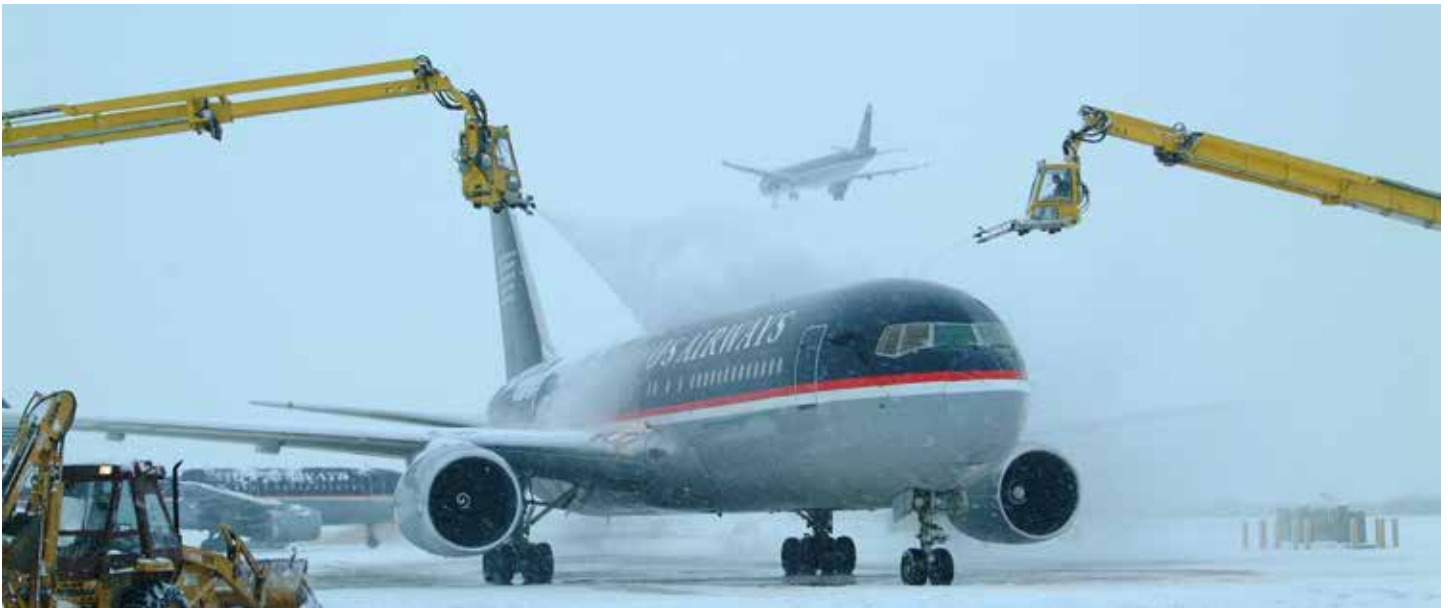
Typical commercial aircraft being deiced prior to takeoff (Photo: Rick Mullin).
