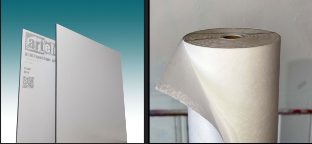
Mural cloth over ACM Panel with two layers of crotech sealant
