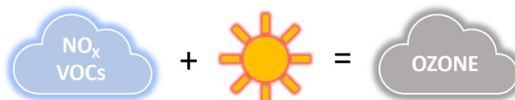
Figure 6. Ozone forms when NO x and VOCs react in sunlight.
