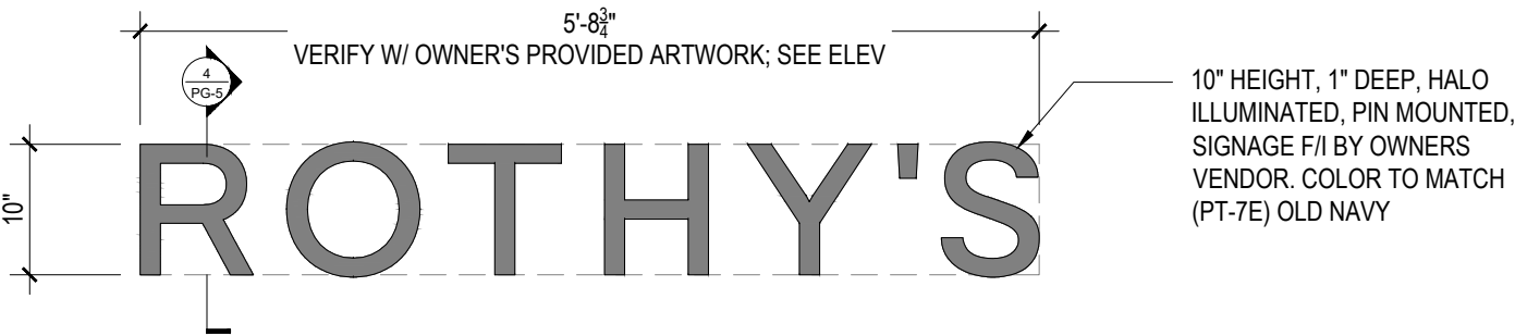
3 HALO LIT SIGNET SIGNAGE ELEVATION SCALE: 3/4" = 1'-0"
