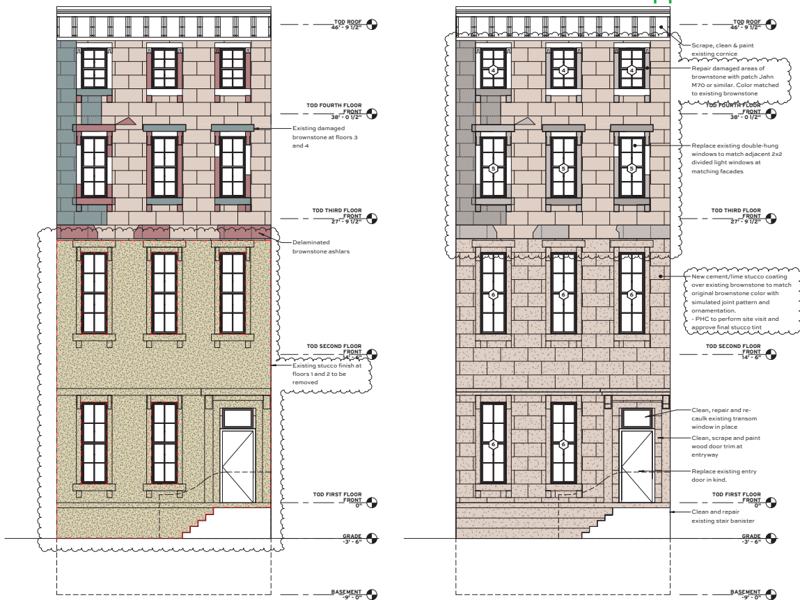
1 PINE ST ELEVATION - EXISTING CONDITIONS H101 1/4" = 1'-0"
