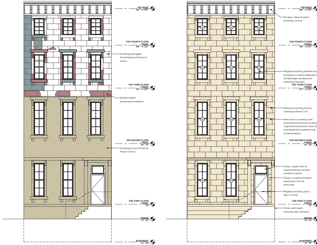
1 PINE ST ELEVATION - EXISTING CONDITIONS 1/4" = 1'-0"
