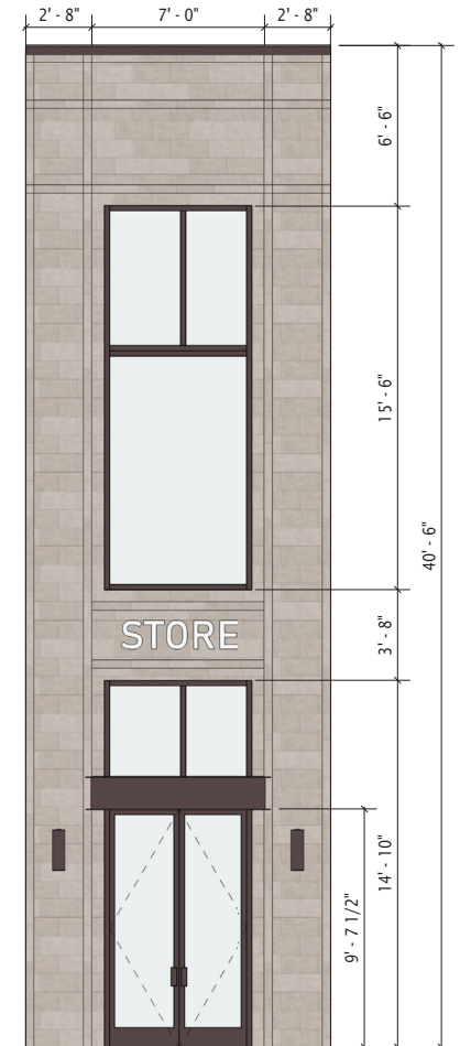
LIMESTONE PIER DETAIL SCALE: 3/16" = 1'-0"
