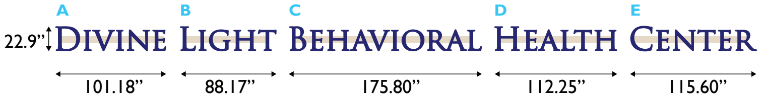
Front-lit Plex Face Channel Letters w/LED - Raceway Mounted - Divine light B.H.C.
