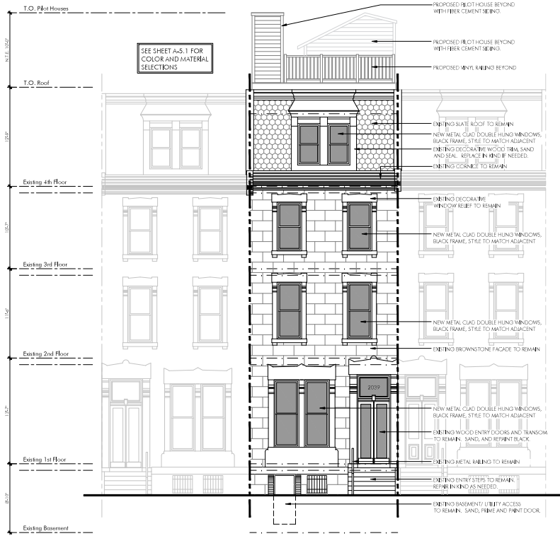
1 Proposed Front Elevation Scale: 3/16" = 1'-0"
