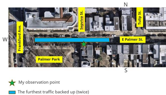
Figure 7: Visualization of furthest queue length on Palmer Street from Frankford Avenue to Tulip Street
