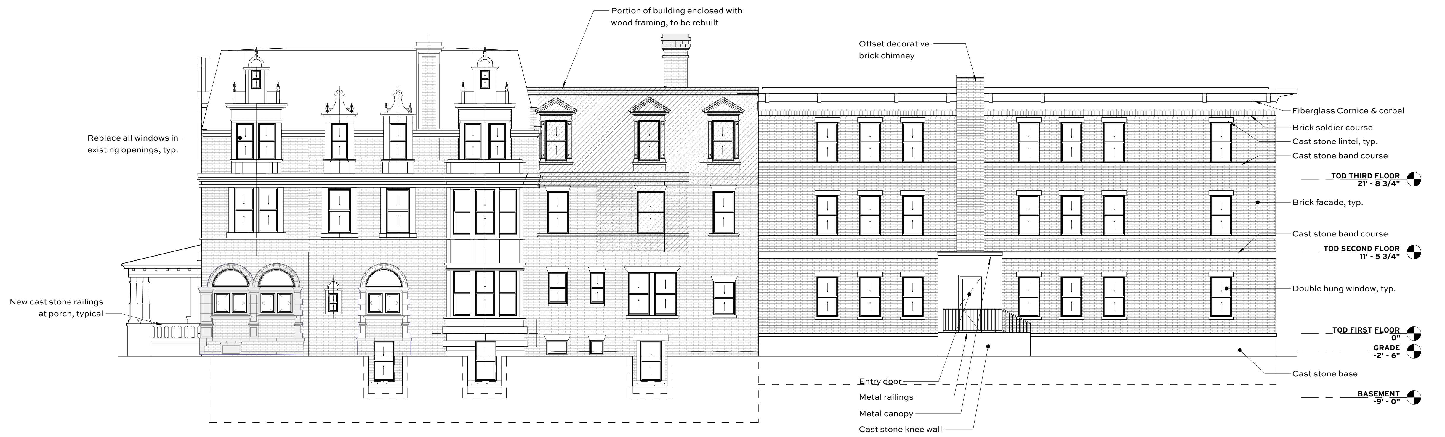
6 SCHEMATIC EAST ELEVATION H105 1/8" = 1'-0"
