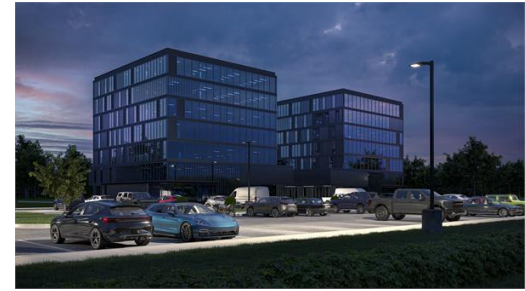
25' TALL LIGHTPOLES WITH FULL-CUTOFF LED AREA LIGHTS
