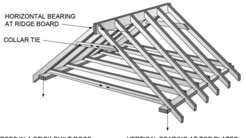
FORCES IN A STICK-BUILT ROOF
