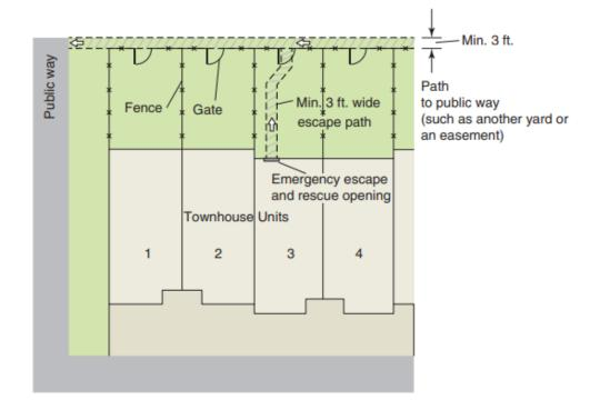
**R310.1 Emergency escape and rescue opening required.** Basements, habitable attics and every sleeping room shall have not less than one operable emergency escape and rescue opening. Where basements contain one or more sleeping rooms, an emergency escape and rescue opening shall be required in each sleeping room. Emergency escape and rescue openings shall open directly into a public way, or to a yard or court having a minimum width of 36 inches (914 mm) that opens to a public way.
