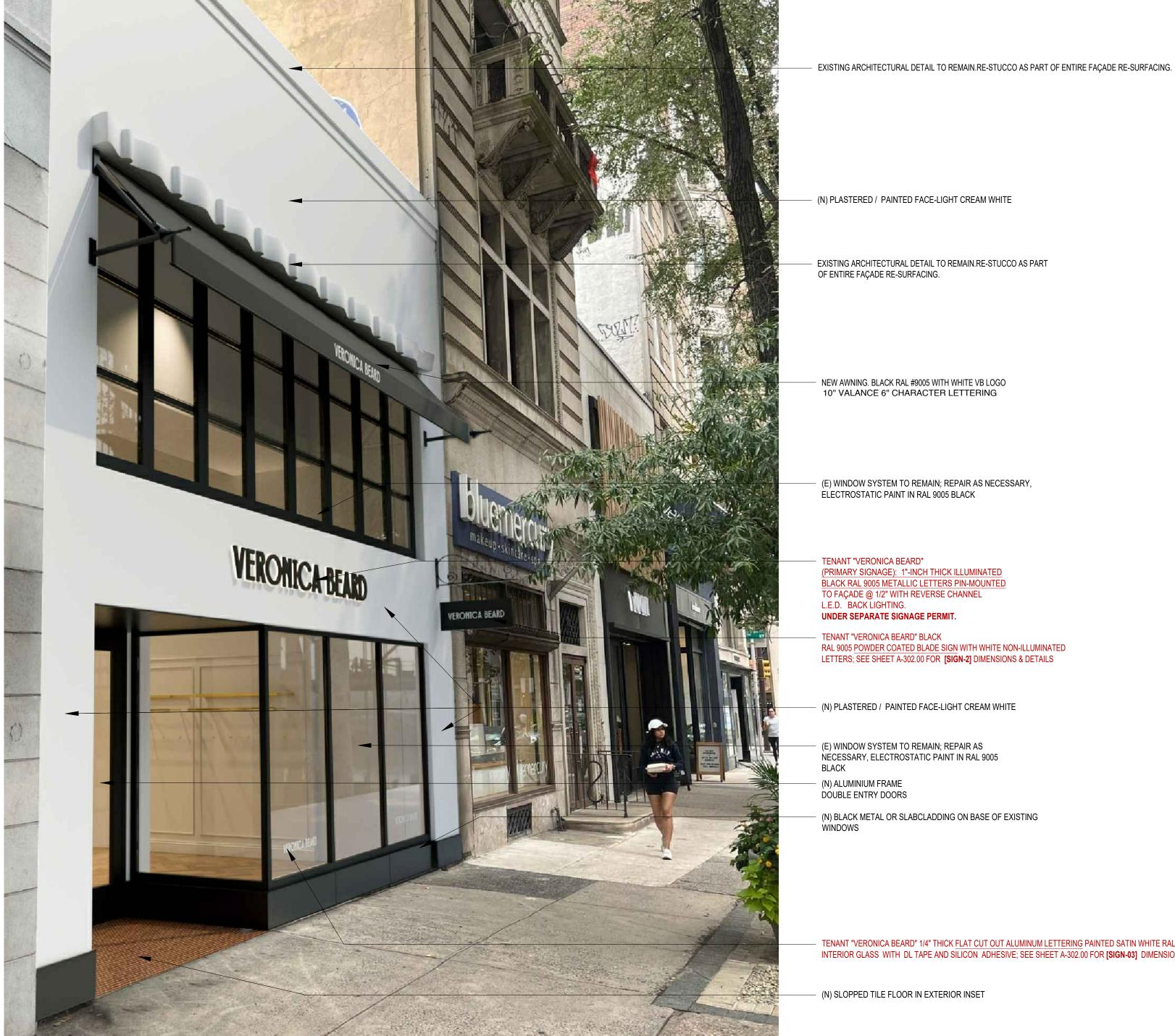
(N) PLASTERED / PAINTED FACE-LIGHT CREAM WHITE EXISTING ARCHITECTURAL DETAIL TO REMAIN.RE-STUCCO AS PART OF ENTIRE FAÇADE RE-SURFACING. NEW AWNING. BLACK RAL #9005 WITH WHITE VB LOGO 10" VALANCE 6" CHARACTER LETTERING (E) WINDOW SYSTEM TO REMAIN; REPAIR AS NECESSARY, ELECTROSTATIC PAINT IN RAL 9005 BLACK (PRIMARY SIGNAGE): 1"-INCH THICK ILLUMINATED BLACK RAL 9005 METALLIC LETTERS PIN-MOUNTED TO FAÇADE @ 1/2" WITH REVERSE CHANNEL L.E.D. BACK LIGHTING. **UNDER SEPARATE SIGNAGE PERMIT.**
