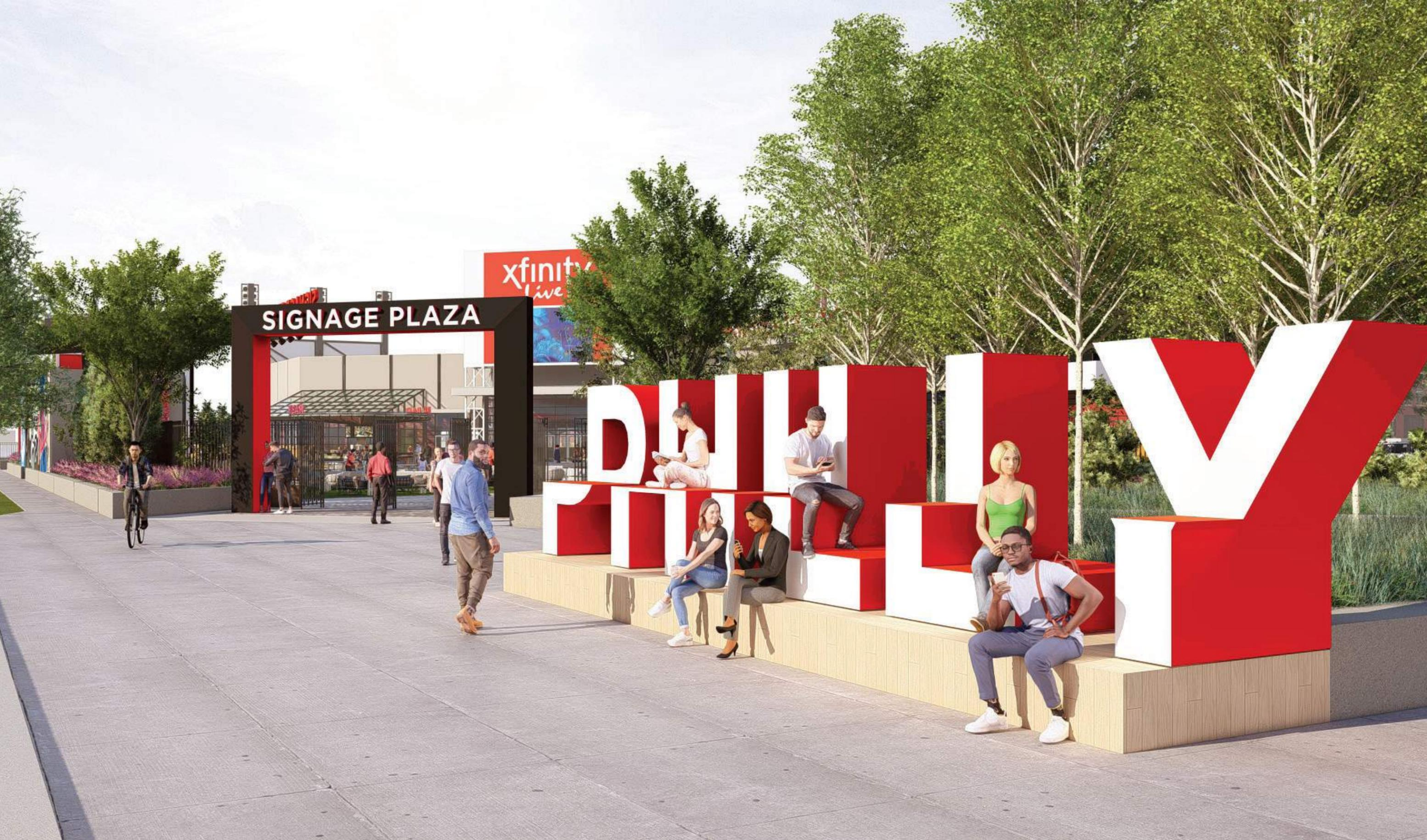
**A01** Aluminum channel letters with acrylic face, decorative face trim, and painted trim and returns. Illuminated via white LEDs. Mounted to painted external signage support frame/raceway. Internally illuminated.
