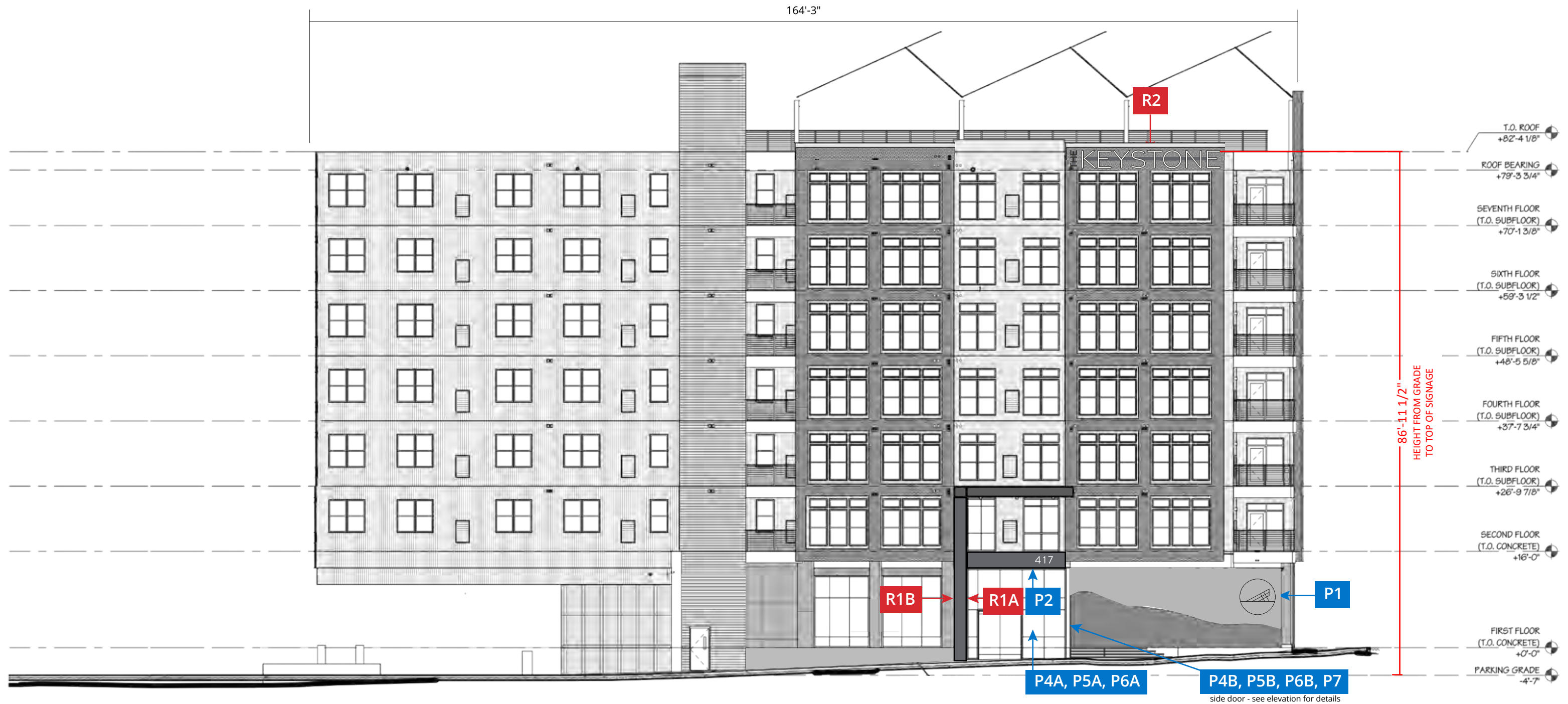
1 West Elevation Scale: 1/16" = 1'
