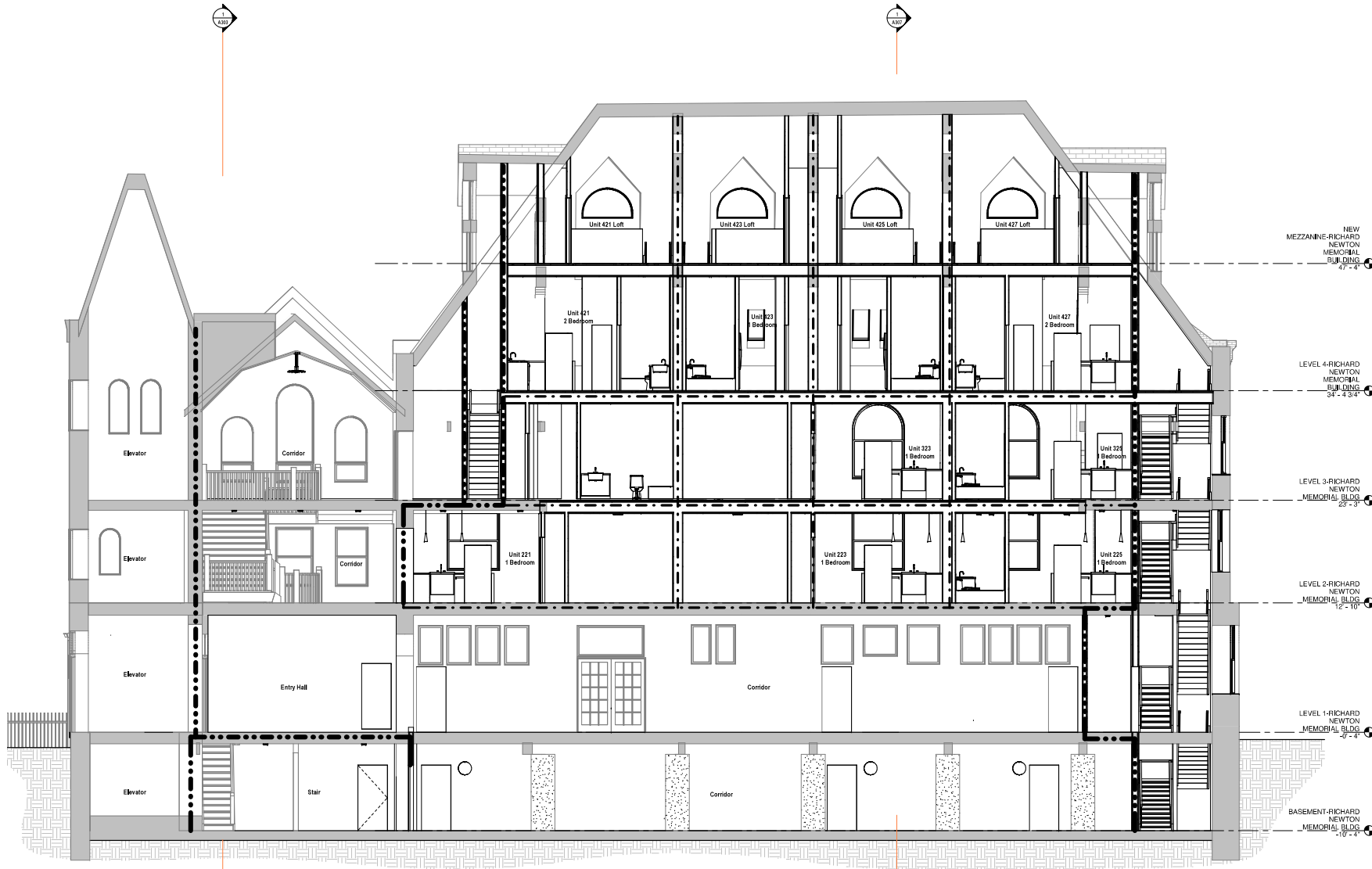
A304 Longitudinal Section Through Richard Newton Building 1/8" = 1'-0"
