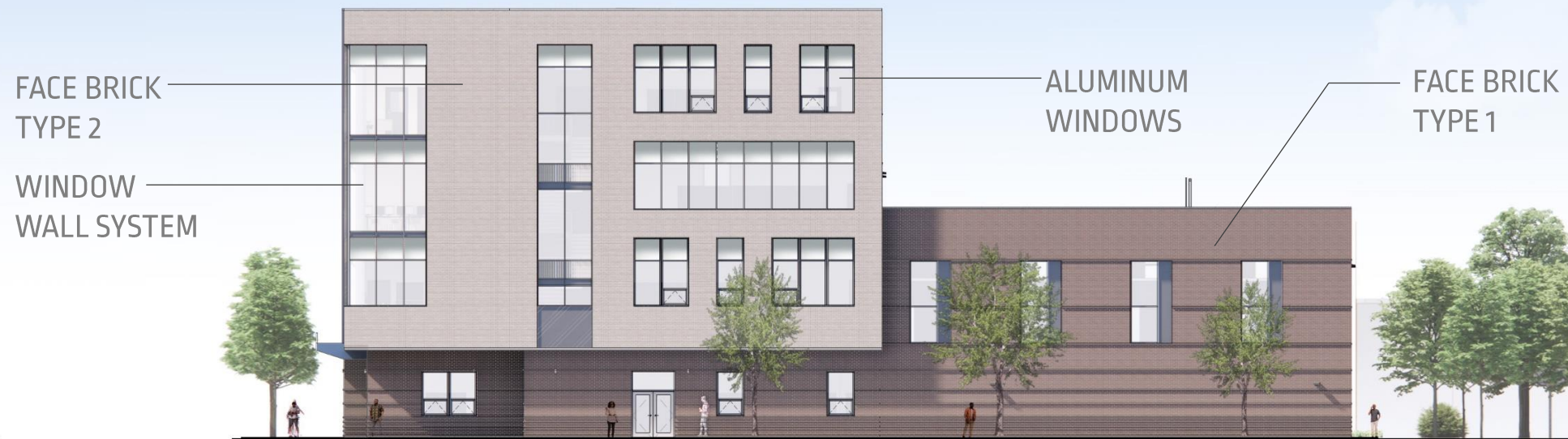
2 EAST ELEVATION – E ONTARIO ST
