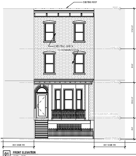
01 FRONT ELEVATION 3'-10" x 14'-0"
