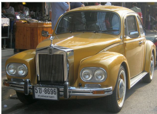
Modified Volkswagen as Rolls Royce – disparate parts but VW windshield and rear volume. It is not a Rolls.
