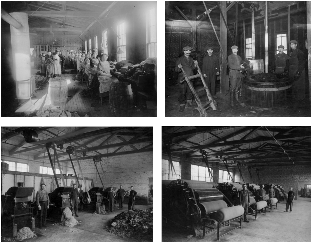
Figure 5: Interior views of the Slack Shoddy Mill in Springfield, Vermont. The interior of the Keystone Mill during the tenure of William Johnston & Sons would have been very similar in appearance. Clockwise from top left, these images depict the sorting, scouring, picking, and carding processes (from slackshoddimill.com).
