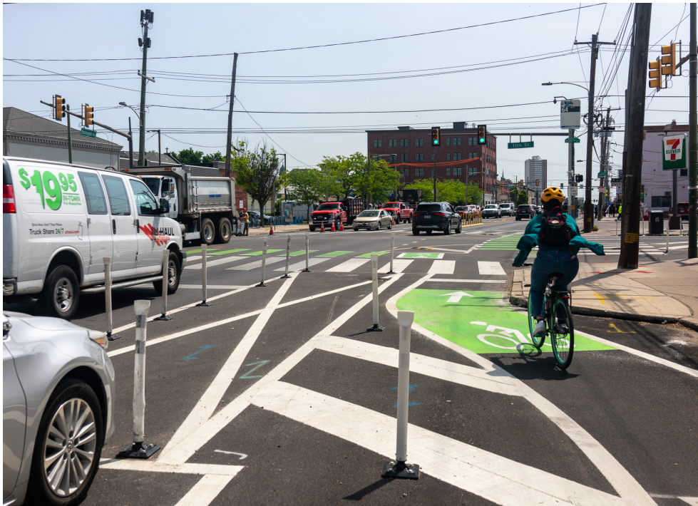
Above: A person riding a bicycle on Washington Avenue at 11 th Street, using the new parking-separated bicycle facility
