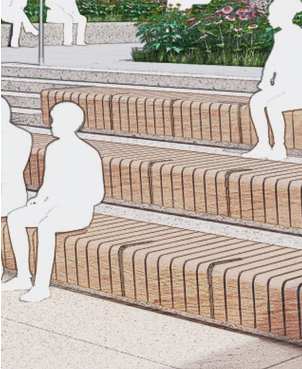
Wood seat tops with integral fins on existing granite stairs
