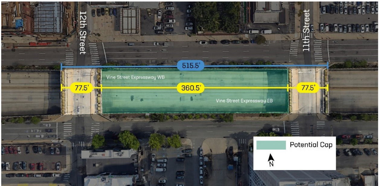
Figure 4: Measurements from 11th Street Bridge to 12th Street Bridge
