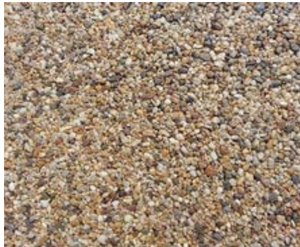
BONDED AGGREGATE - POROUS
