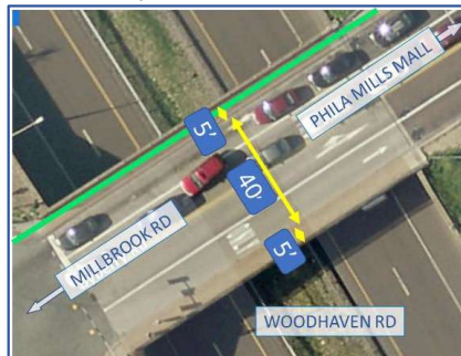
Alternative B trail overpass has very little room to accommodate bikes and pedestrians.
