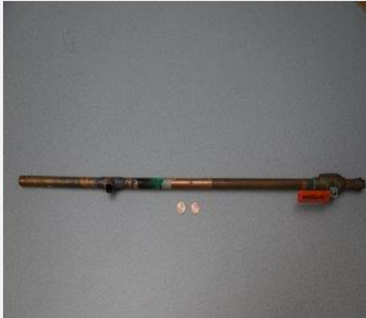
Copper pipe, scratched by coin
