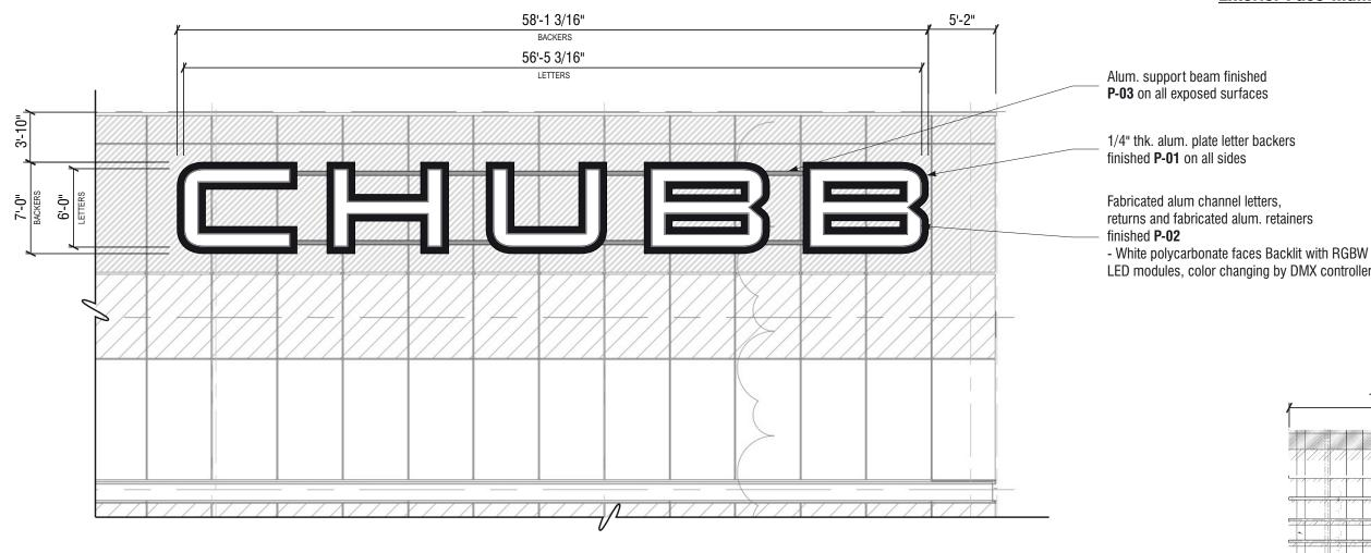
**Sign 4** - West Elevation (20th Street) - Detail Scale: 1/8"=1'-0"
