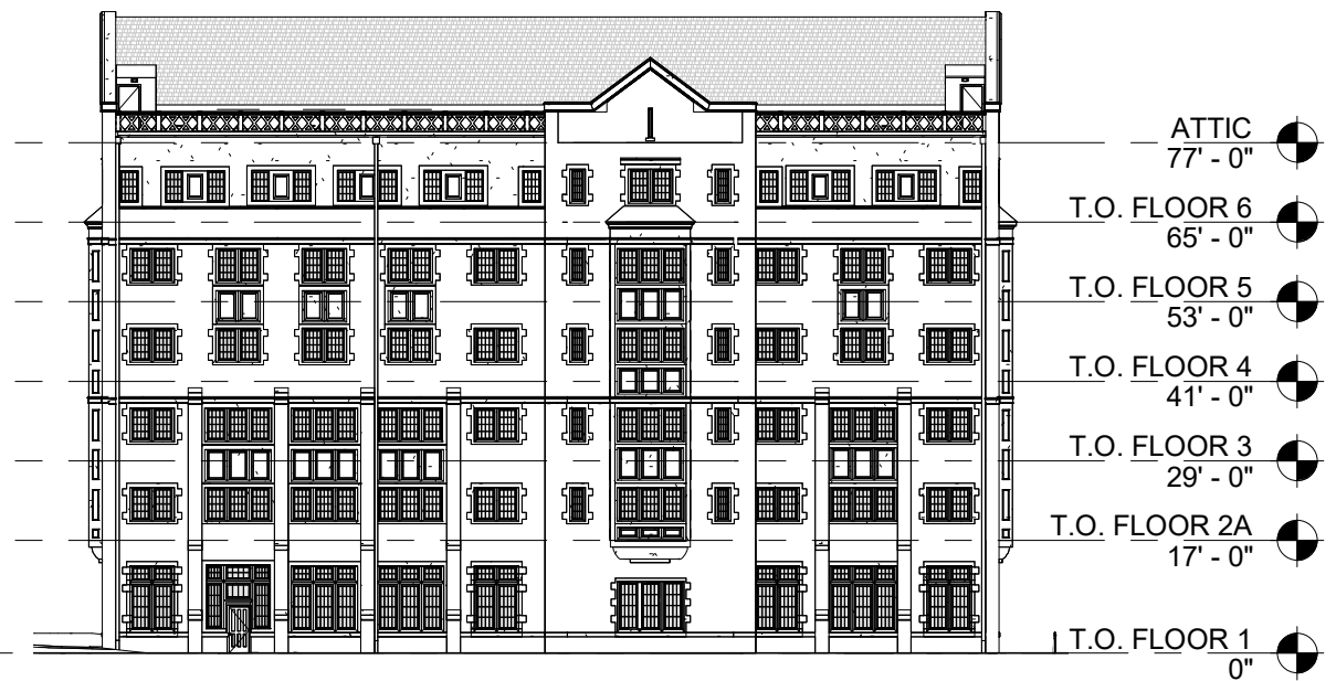
1 SOUTH ELEVATION AT SERVICE ROAD 1/32" = 1'-0"
