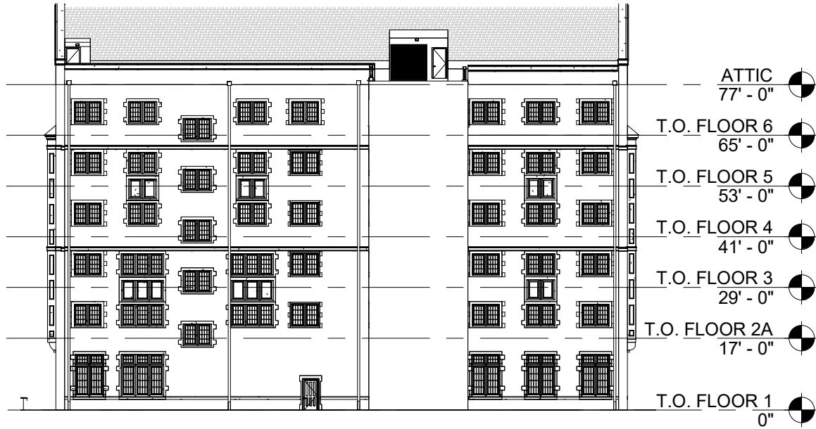
5 ELEVATION AT NORTH SIDE OF CARDINAL ARCHWAY 1/32" = 1'-0"
