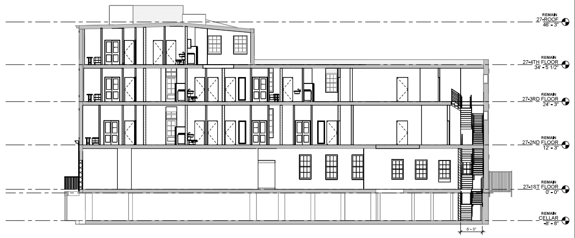
3 BLDG 27 LONG SECTION, PROPOSED 1/8" = 1'-0"
