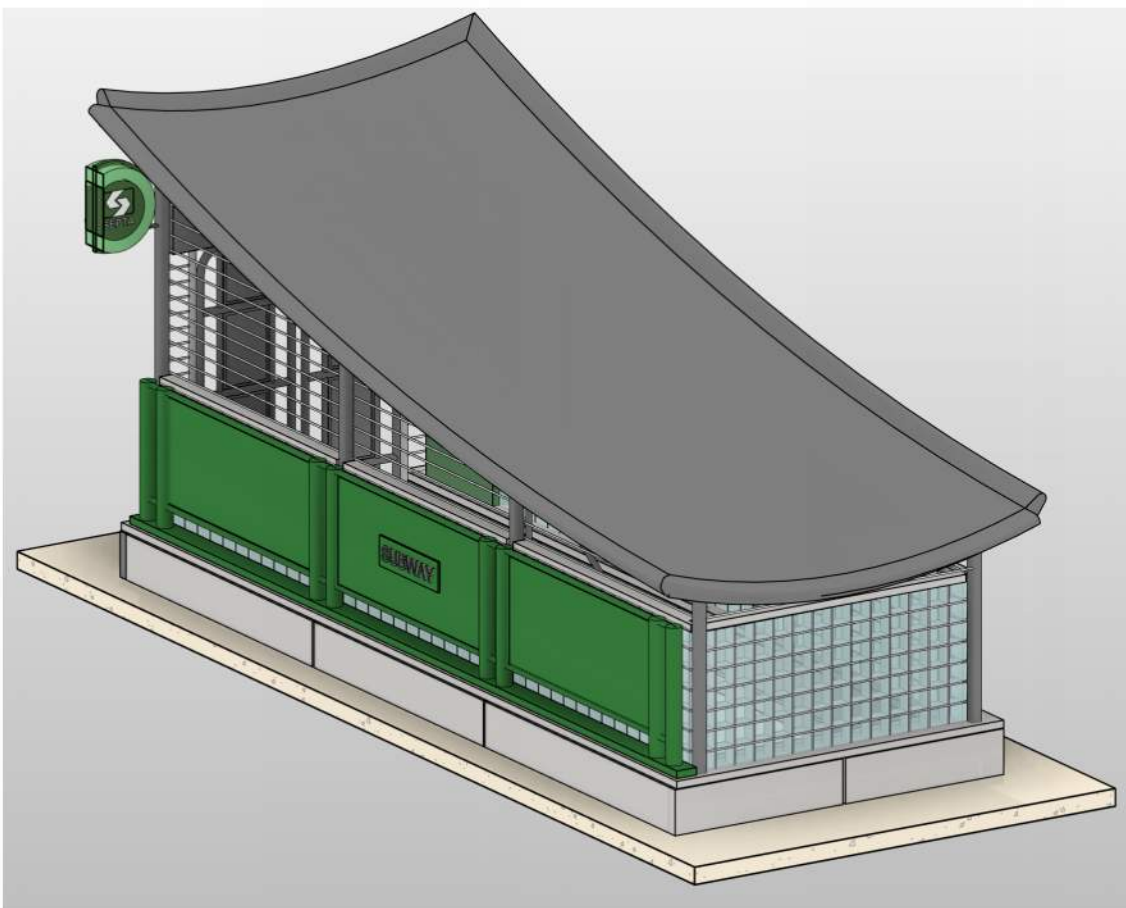
② 3D VIEW OF STAIR HEADHOUSE CONCEPT
