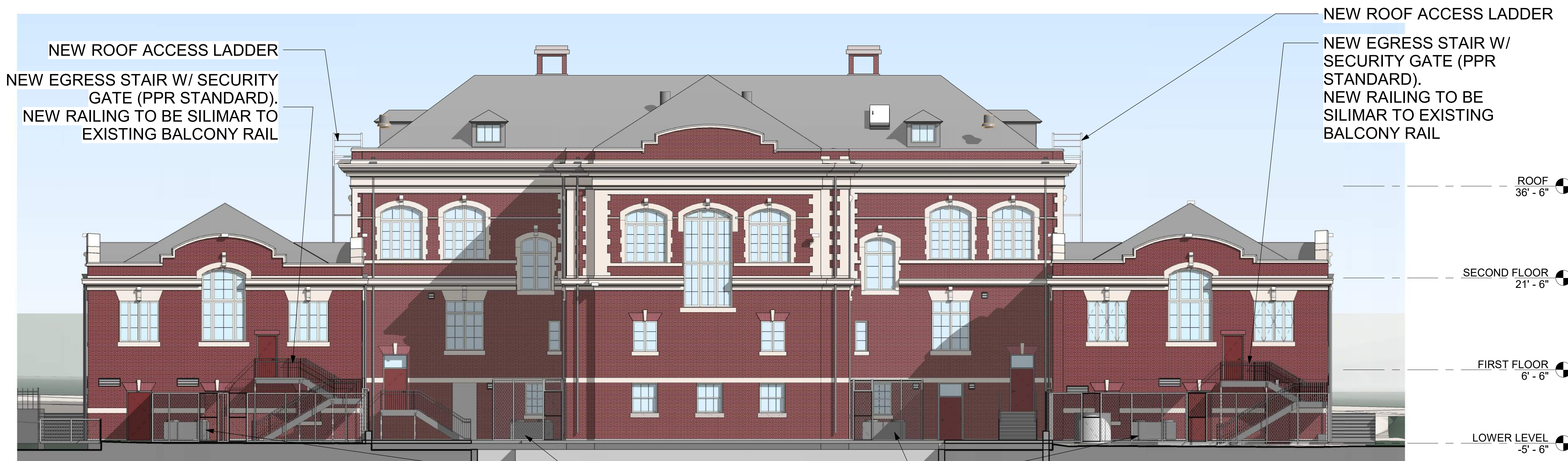
WEST ELEVATION - POOL SIDE
