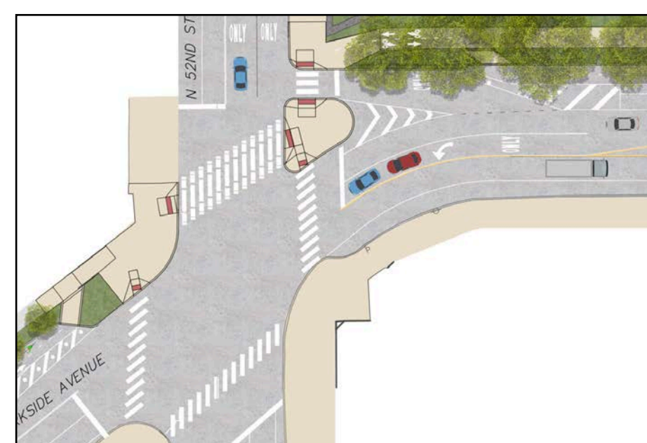
3. Intersection Improvements with new concrete bus boarding islands, pedestrian islands, and concrete bumpouts
