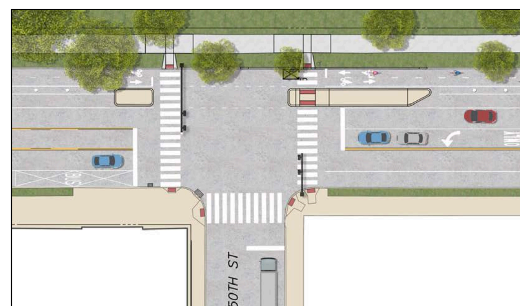
3. Intersection Improvements with new concrete bus boarding islands, pedestrian islands, and concrete bumpouts
