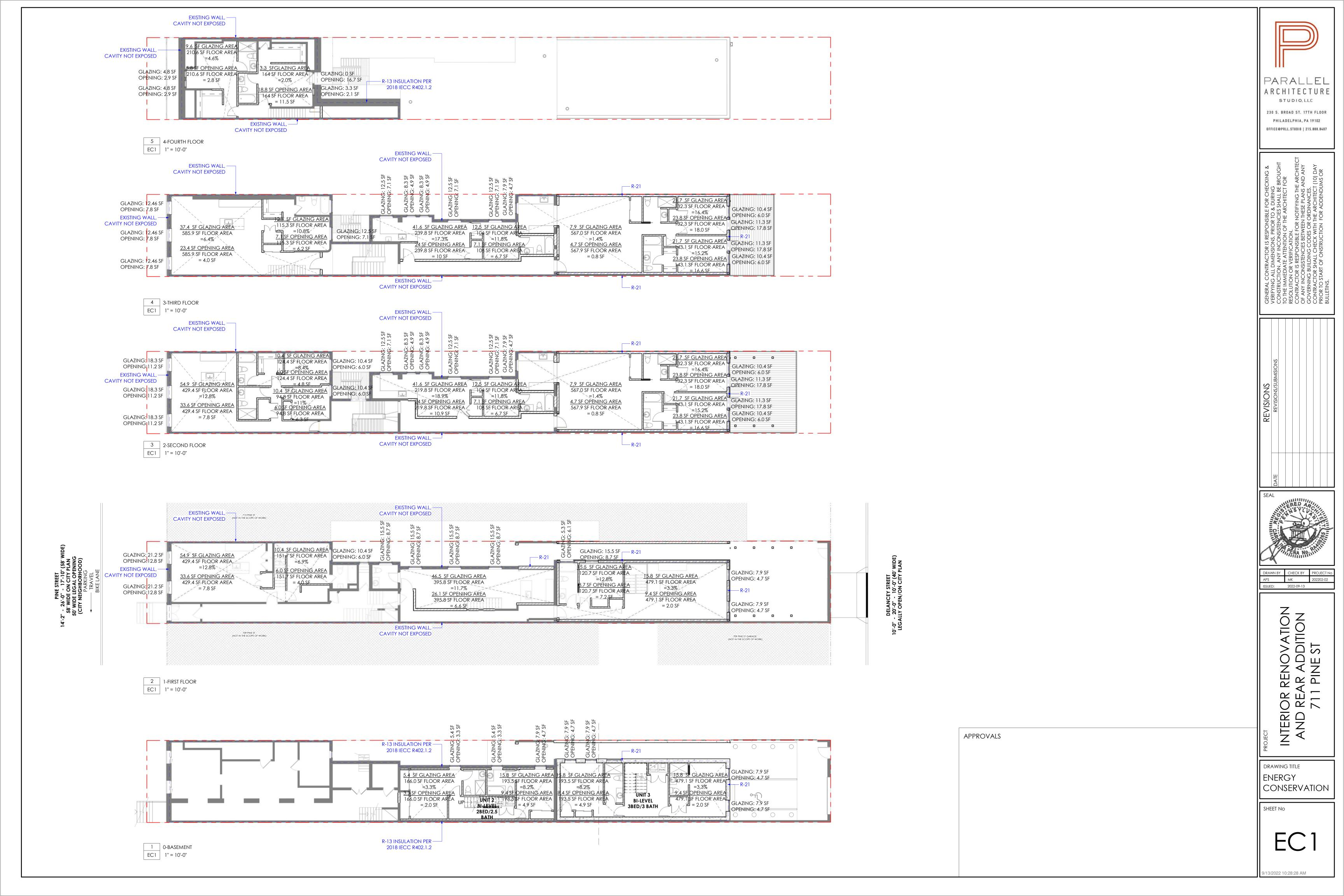
ROOF 56' - 4" -R-38 INSULATION R-38 INSULATION 4.0 4TH FLOOR FRONT 41' - 4" R-38 INSULATION R-38 INSULATION 3.2-3RD ROOF REAR 35' - 2" EXISTING WALL, — CAVITY NOT EXPOSED R-21 INSULATION 1.0-1ST FLOOR FRONT 4' - 6" 1.0-1ST FLOOR FRONT 4' - 6" 0.1-BASEMENT REAR -2' - 6" 0.1-BASEMENT REAR -2' - 6"\_\_\_\_\_\_ 1 Section EC EC2 1/8" = 1'-0"
