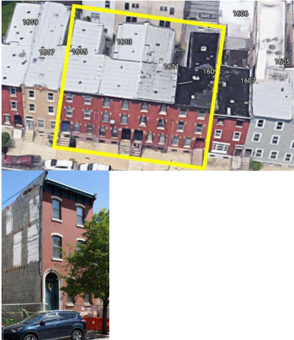
Figure 4. (L) An aerial image of the north side of the 1600 block of Christian Street shows the L-shaped plan of each row and the typical ABAB pattern of arrangement (image by Google Earth). (R) 1625 Christian Street (Image by Adrian Trevisan)
