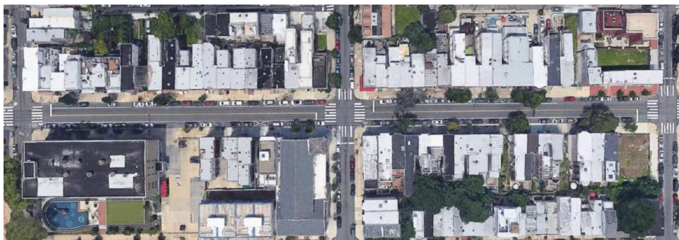
Figure 11. Aerial image of the 1500 and 1600 blocks of Christian Street. The L-shaped layout of the rows on the north side of the street most resemble Plan C. In elevation, most Christian street row houses resemble the simple facade of Plan A (Google Earth).
