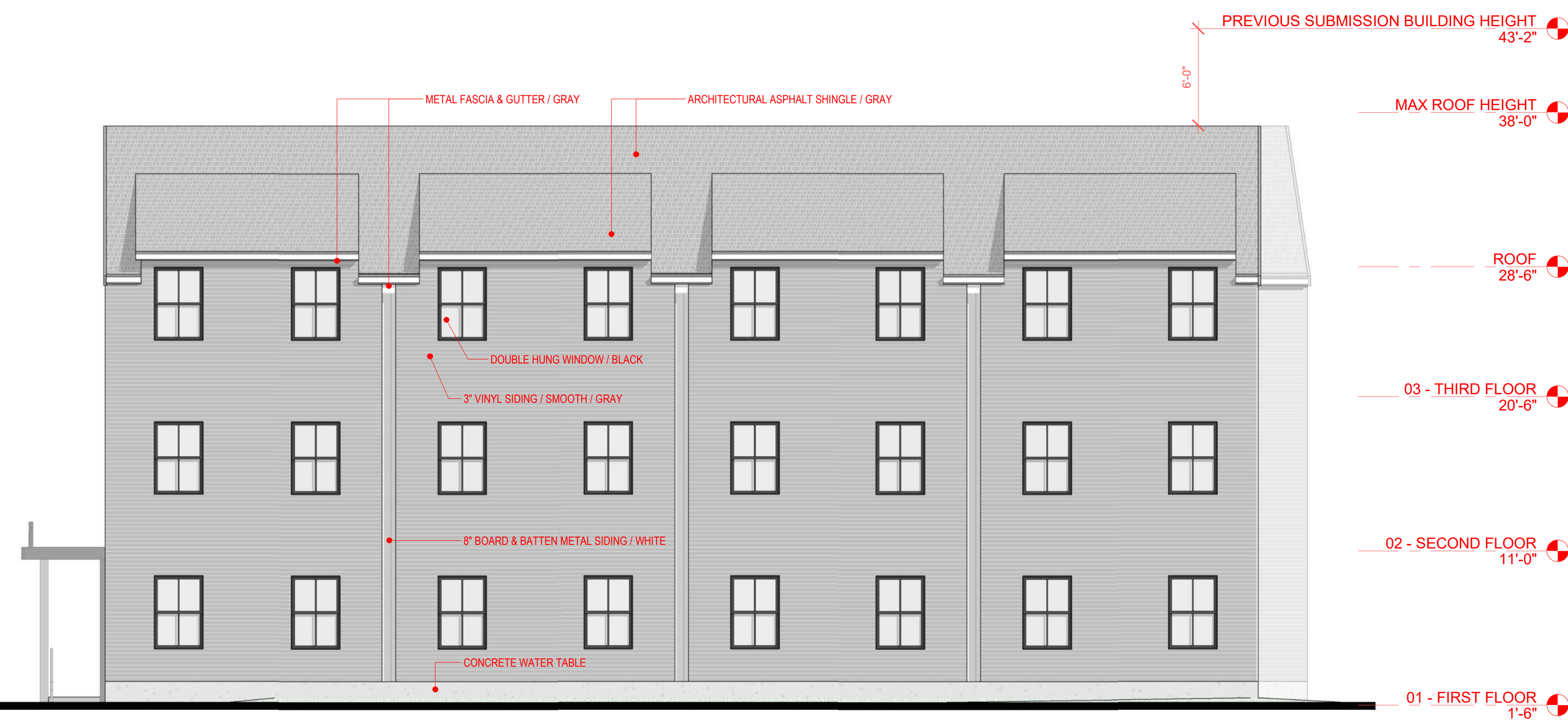
4 PROPOSED BUILDING - SIDE ELEVATION 02 3/16" = 1'-0"
