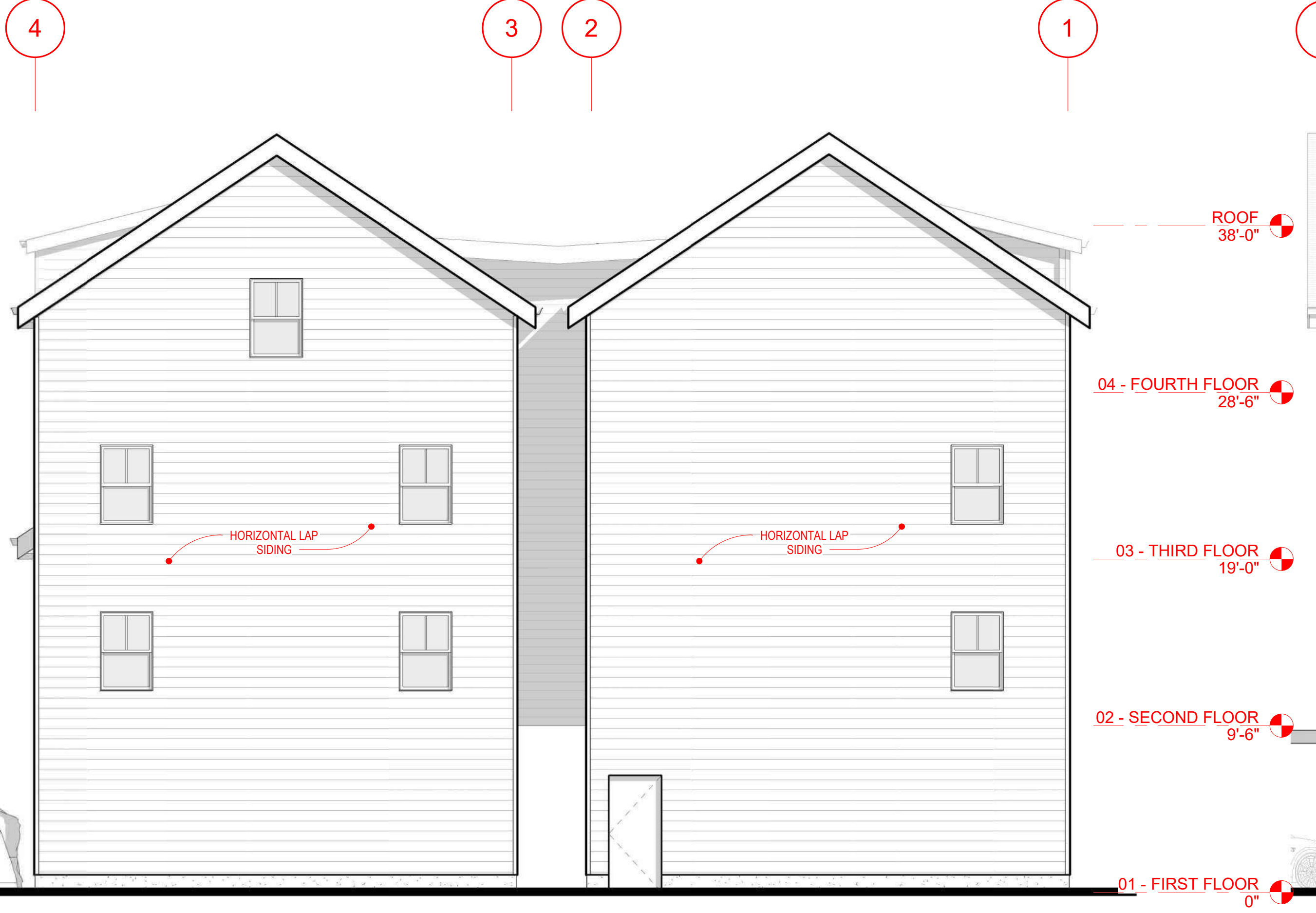
3 PROPOSED BUILDING - REAR ELEVATION 3/16" = 1'-0"
