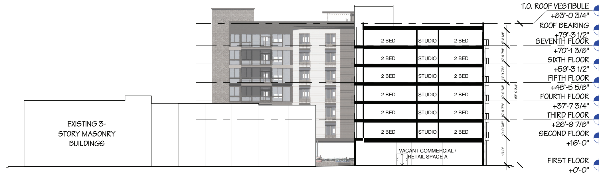
2 NORTH-SOUTH BUILDING SECTION SCALE 1/32" = 1'-0"
