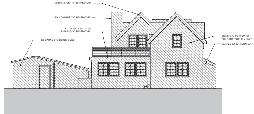
SOUTH ELEVATION - EXISTING - 3 Dependent 1 A-300 / 3/16" = 1'-0"
