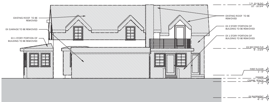
WEST ELEVATION - EXISTING - 2 Dependent 1 A-300 / 3/16" = 1'-0"
