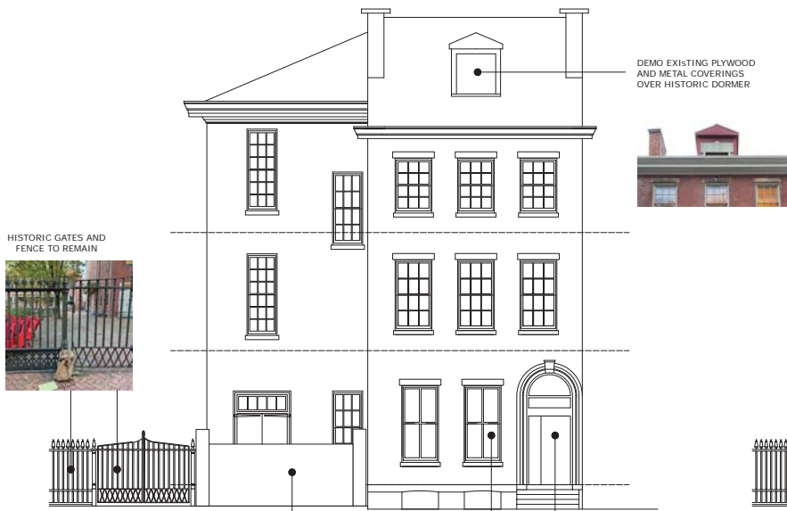
EXISTING North Elevation 3/16" = 1'-0"
