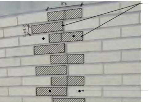
AT EXG CORNERS, CAREFULLY REMOVE BRICKS ADJACENT TO EXG LARGE CRACKS (GREATER THAN 1/16") WHERE THE BRICK HAS SEPARATED, SALVAGING UNDAMAGED BRICK UNITS.
