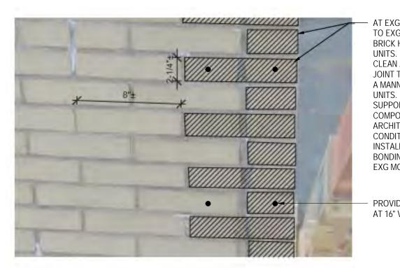
AT EXG CORNERS, CAREFULLY REMOVE BRICKS ADJACENT TO EXG LARGE CRACKS (GREATER THAN 1/16") WHERE THE BRICK HAS SEPARATED, SALVAGING UNDAMAGED BRICK
