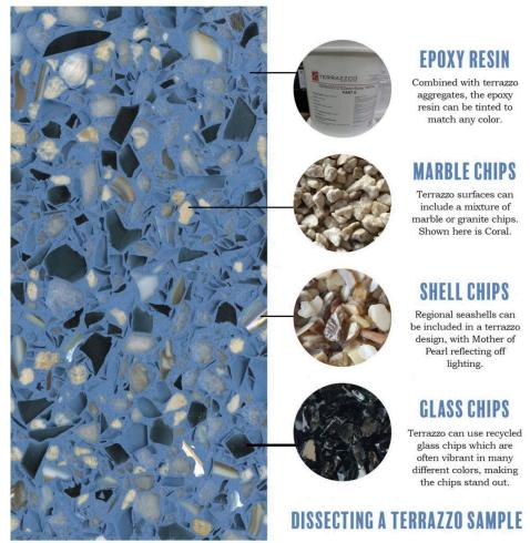
Terrazzo or polished concrete is an ancient and durable material. It is often used as a flooring in public spaces. Terrazzo allows for metal inlay as well as a huge array of colors and aggregates. The capstones will be a rainbow of different colored concrete that is polished to expose a brass inlay.
