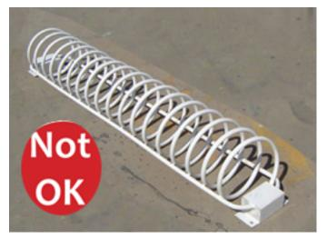
This bike rack does not meet the minimum standards listed on the previous page. Because the bike rack structure is short, it cannot support an upright bicycle in two places. Due to its low-to-the-ground design, it does not enable a bicycle's frame and at least one wheel to be locked to it. Additionally, this bike rack is a trip hazard for pedestrians.
