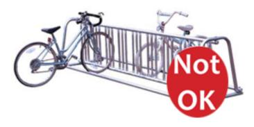
This bike rack does not meet the minimum standards listed on the previous page. This bike rack exceeds the 42" maximum length. Additionally, it does not enable a bicycle's frame and at least one wheel to be locked to it.
