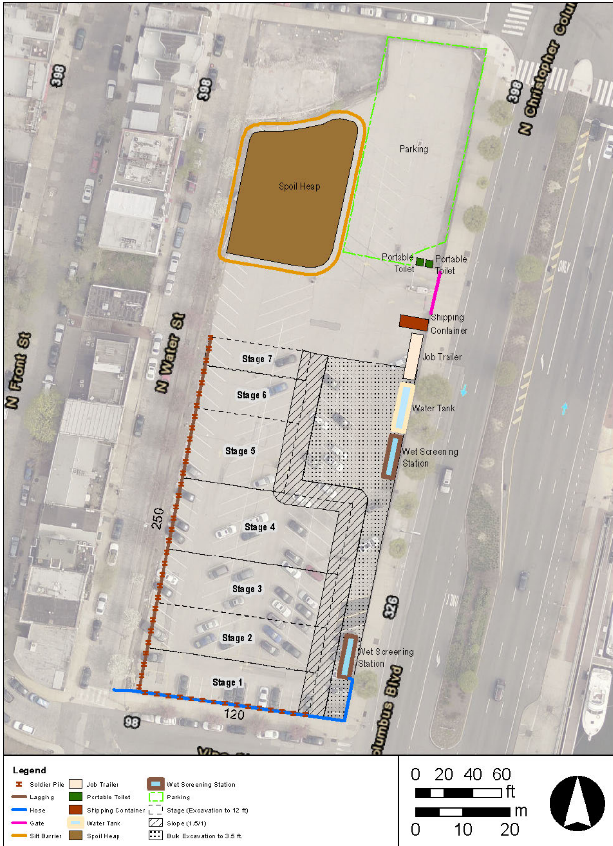
Figure 4. Map of the project area showing the proposed order of excavation and the layout of the site facilities.
