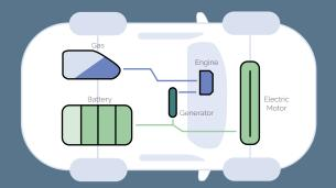
PHEVs can be powered by an internal combustion engine that can run on conventional or alternative fuel and an electric motor that uses energy stored in a battery. The vehicle can be plugged in to an electric power source to charge.
