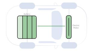
All-electric vehicles, also known as BEVs, rely solely on electric motors to make them go. Large batteries give them longer range. They need to be plugged into a power source to charge.
