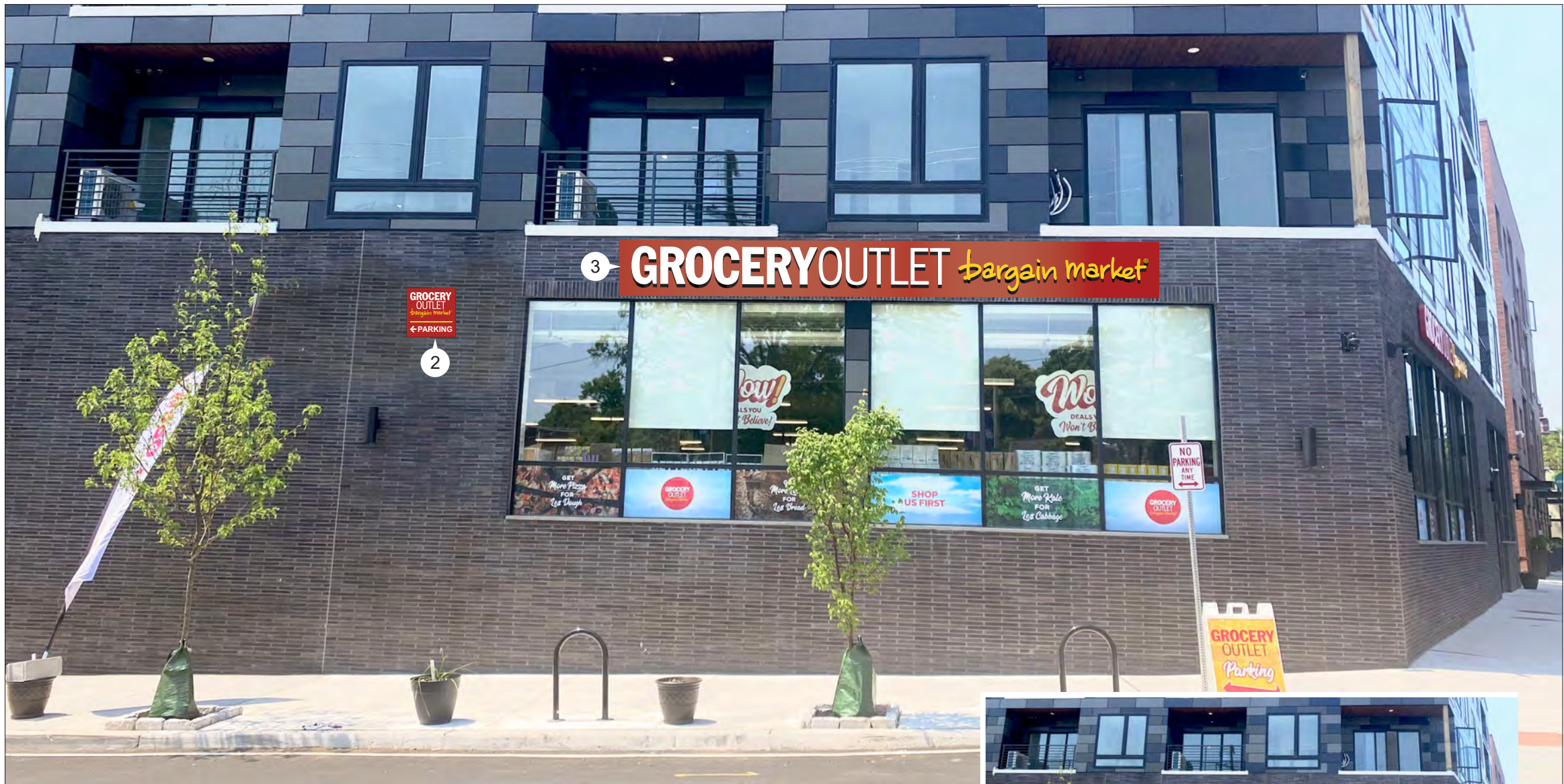
W HORTTER ST @ CORNER Sign Type (2) (QTY:1) Illuminated wall mount sign. Sign Type (3) (QTY:1) Pan mounted channel letters sign. Scale: NTS
