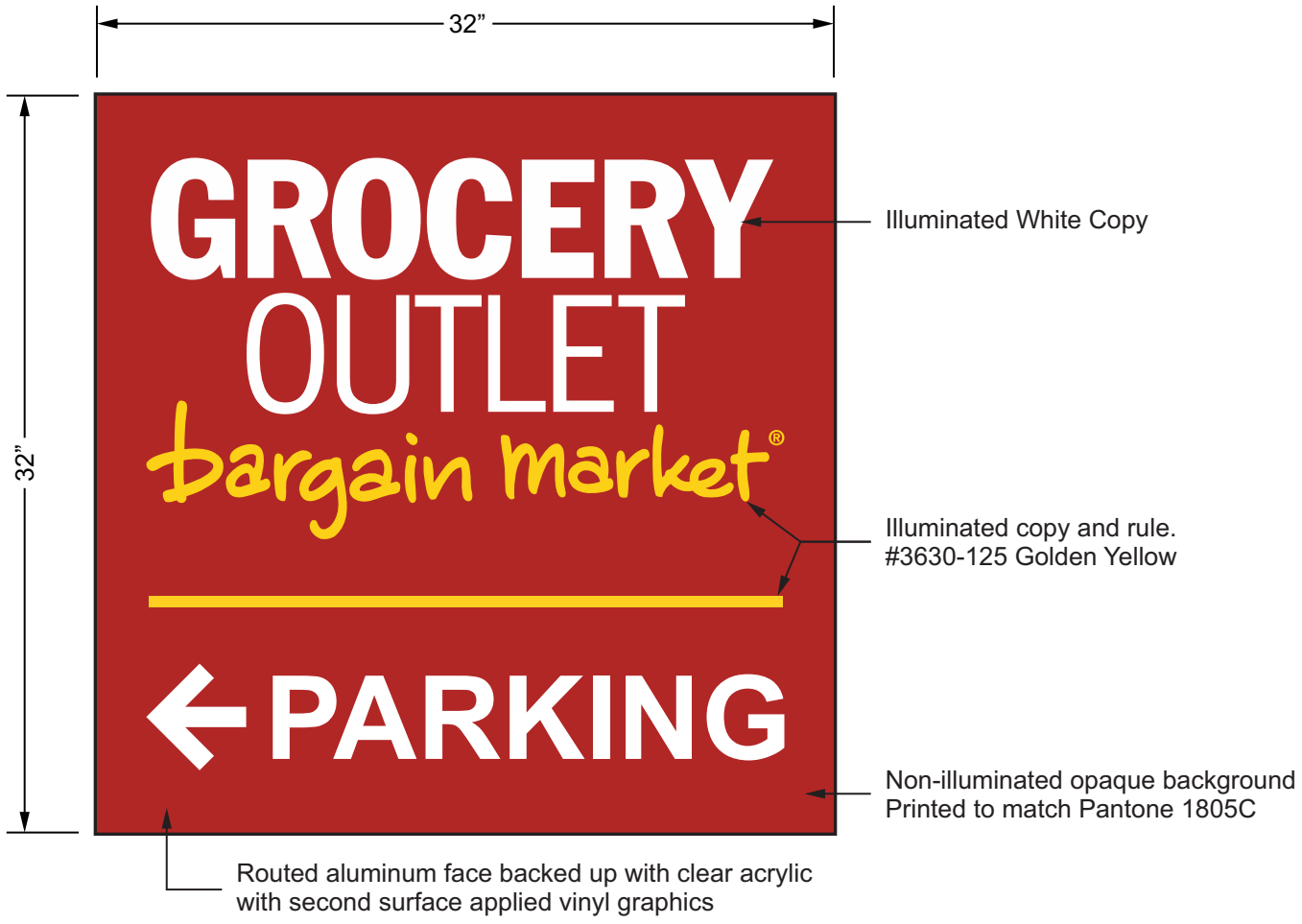
SIGN ELEVATION - Sign Type (2) (QTY:1) Illuminated wall mount sign. Scale: 1:8 (7.11 SQFT)
