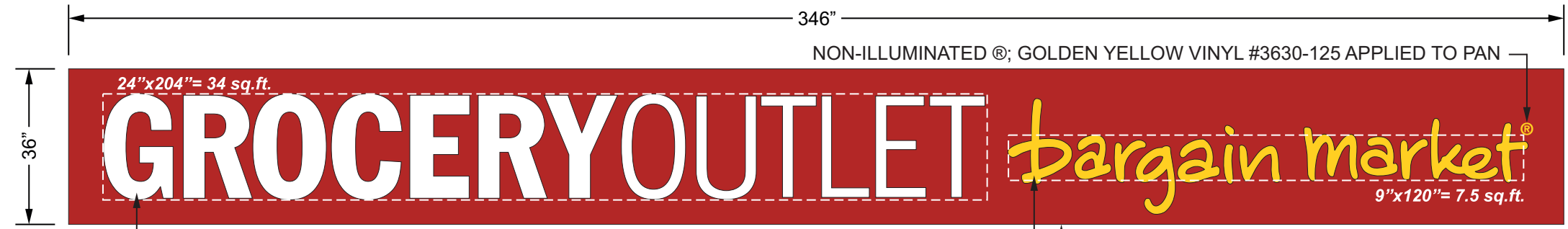
Configuration of Sign Types (4,5,6) - Pan Mounted Channel Letters - Scale: 3/16" = 1'
