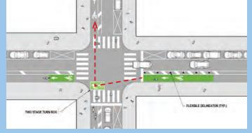
Two-stage turn boxes offer people on bikes a safer way to make turns at cross intersections. Adding these boxes at key locations on Spruce and Pine will give people on bicycles a visible path across the intersection without the need to merge with or cross vehicle traffic.
