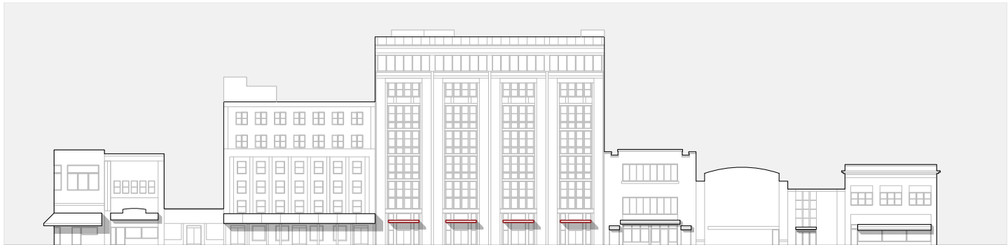
DESIGN SOLUTION: INTRODUCE ORDERLY HORIZONTAL ELEMENTS
