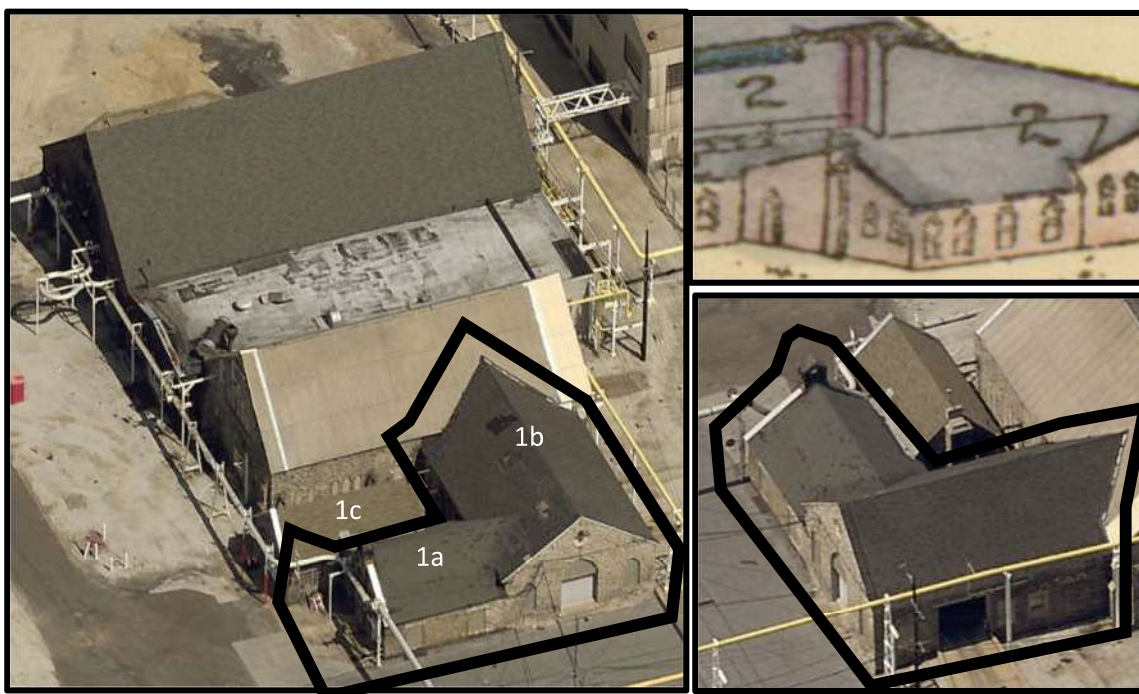
Figure 8. Left: Looking north at Resource Nos. 1—1a, 1b, and 1c, 2, and 5—5a and 5b, showing, specifically, Resource Nos. 1a, 1b, and 1c. The original portion of Resource No. 1: Purifying House (1853–54) is delineated in black. Source: Atlas, City of Philadelphia, 2018. Figure 9. Top right: 1894 Hexamer General Survey of the Point Breeze Gas Works, showing, specifically, Resource No. 1c (labeled 2 in the Hexamer) of the larger building. Source: Greater Philadelphia GeoHistory Network. Figure 10. Bottom right: Looking northwest at Resource No. 1: Purifying House (1853–54), showing, specifically, Resource Nos. 1a, 1b, and 1c. The original portion of Resource No. 1: Purifying House (1853–54) is delineated in black. Source: Atlas, City of Philadelphia, 2018.
