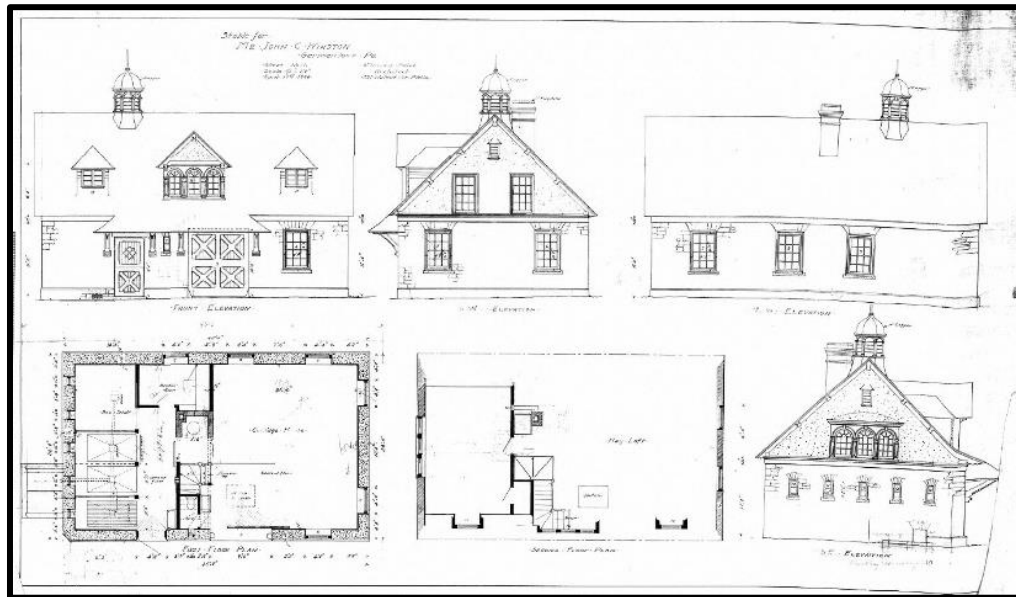
Figure 56. Plans and Elevations of John C. Winston's Stable at 5208 Wayne Avenue in Germantown, dated 17 April 1900, by William L. Price, architect. Source: The William L. & Walter F. Price Collection, Athenæum of Philadelphia.
