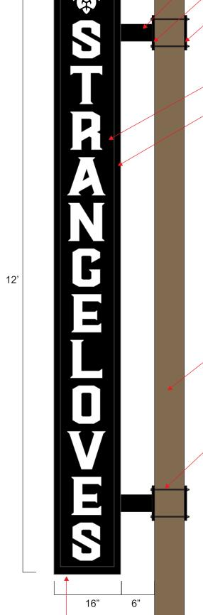
4" ALUMINUM SQUARE TUBE 1/2" THICK ALUMINUM PLATE 8"x 8" SANDWICHED FRONT AND BACK OF EXISTING WALL 3/16" THICK LEXAN FACE BLACK VINYL GRAPHICS
